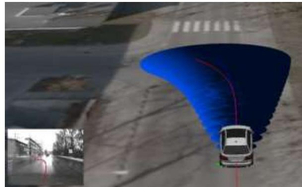
**Fig. 7** Ego-vehicle trajectory prediction using the Trajectory history and present sensor signals like steering angle and yaw rate.
