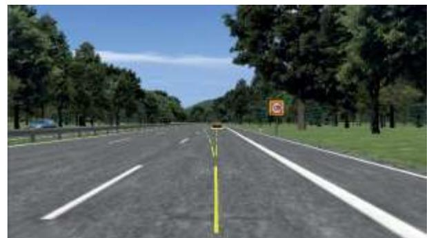
**Fig. 5:** Visualization of intentions (potential trajectories and speed limits) of a highly automated vehicle in a contact-analogue head up display (Damböck et al. 2012b).
