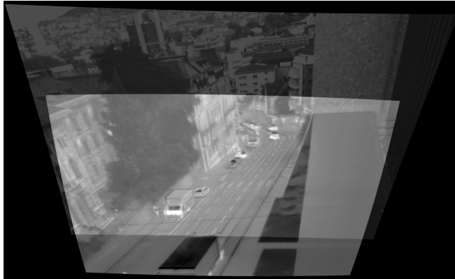
Fig. 5. Image fusion of infrared and visual spectrum image. A pixel mapping based on the assumption of coincident camera centers is used. Images are undistorted and rectified.
