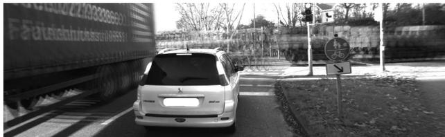
Fig. 1: Moving objects make egomotion estimation difficult.
