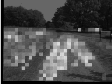
Fig. 6. Brightness-encoded output of the local orientation feature, tested for an orientation of \mu = 0 , i. e. straight ahead. High grayvalues correspond to small orientation differences. Note how the tire marks in the sand cause, in average, significantly larger outputs than the other parts of the image.
