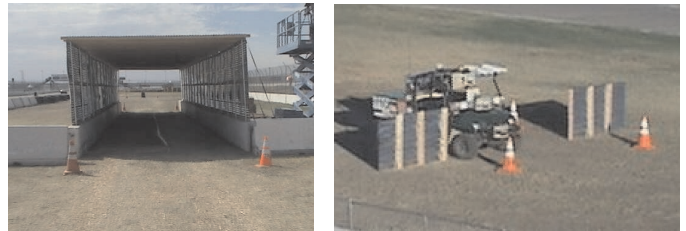
Fig. 1. The Grand Challenge 2005 Qualifying event: The Desert Buceyes autonomous vehicle successfully navigating through a tunnel (left, onboard camera) and a narrow gate bounded by reflecting obstacles (right, spectator's camera).
