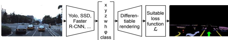
Overview of the intended approach with a camera image and pixel-wise ground truth that is supposed to be used to learn parametric instances, both taken from Apolloscapes dataset.
