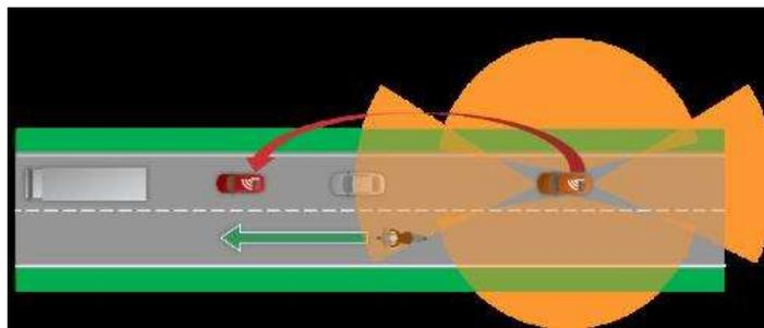
**Fig. 8** Information sharing using Car2x Communication circumvents dangerous situations
