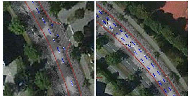
Fig. 7: Results from the mapping process. Detected dashed markings are drawn in blue, road border detections in red.
