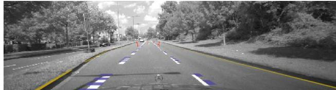
Fig. 1: Map projected into camera image based on current pose determined by our algorithm
