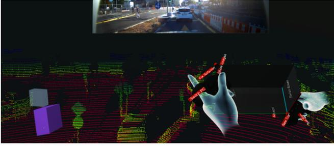
Fig. 3: Tool environment: Point cloud and images are visualized. Two cyclists are labeled. Dummy bounding box between between controllers shall be adopted to the shape of an object.
