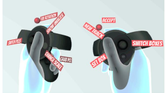
Fig. 4: 3D visualization of the key assignment. Keys on the left controller are used for scene understanding, keys of the right controller are used for data annotation.
