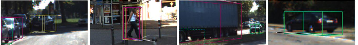
(j) Detailed view of KITTI 3D Ground Truth boxes in KITTI dev kit. Especially boxes in the distance do not match with the ground plane or the real size of the vehicle according to the point cloud. Points outside the box are bright, points inside are dimmed.
