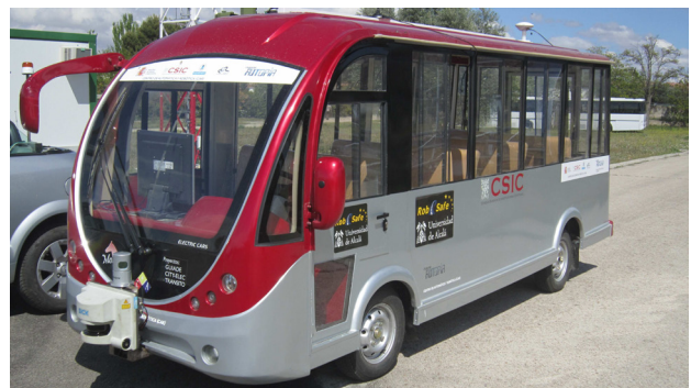
Figure 1. The drive-by-wire electric vehicle used in this experiment has capacity for 14 people. It is equipped with GPS and a multi-beam LIDAR for localization and environment recognition respectively.
