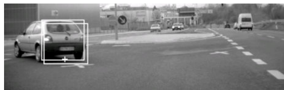
Fig. 4. The target is turning left and is only measured by the camera.
