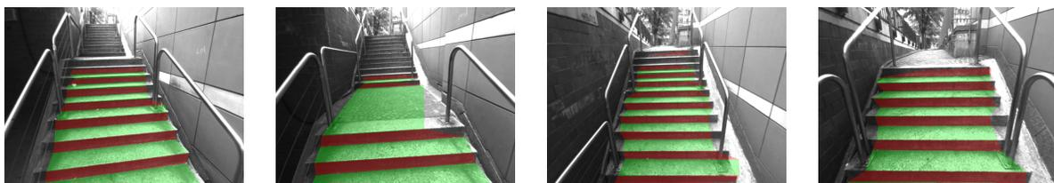
(f) Estimated stair model. Red polygons are detected steps, green polygons connect steps belonging to the same stair.
