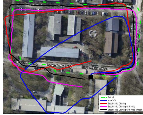
Figure 7: Estimated trajectory for a walk using pure visual odometry (blue) and the stochastic cloning Kalman filter (red). Further improvements are achieved by including measurements of the earth's magnetic field (pink and black). The ground truth is depicted with a green dashed line.
