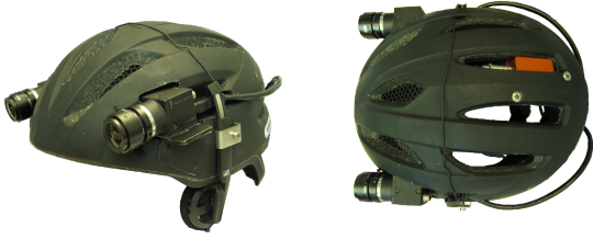
Figure 2: Prototype setup built out of a bicycle helmet, a binocular camera, headphones and an inertial measurement unit (IMU).
